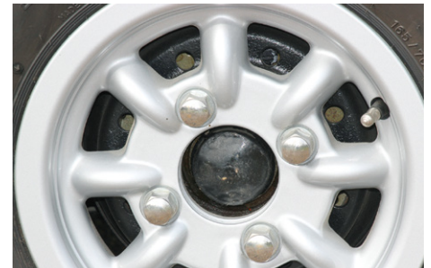
Rear brake drums were drilled.
