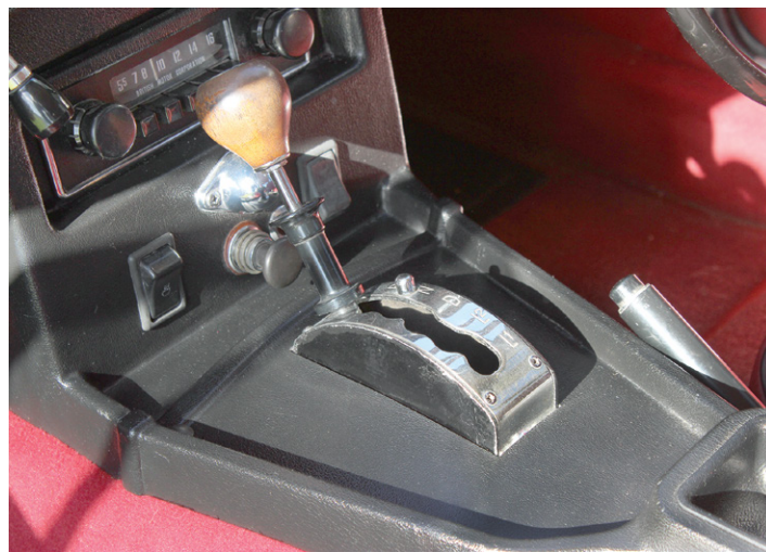
Transmission tunnel was wider to accommodate Borg Warner auto.
