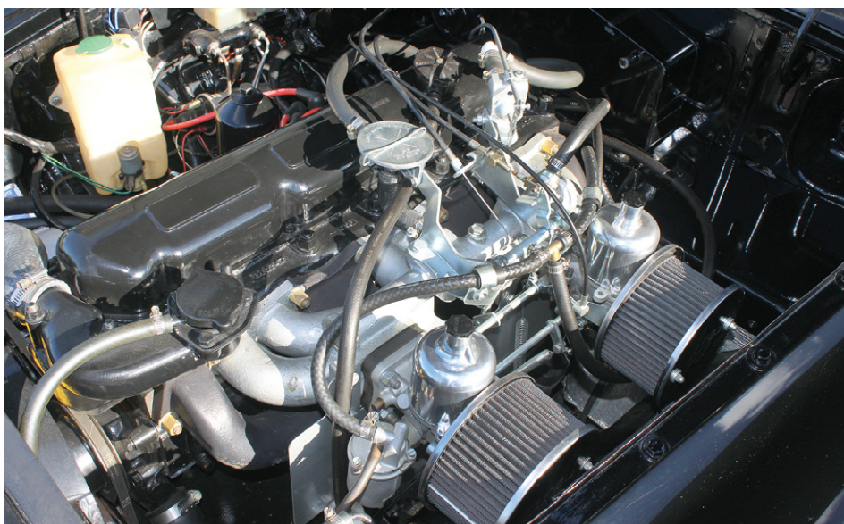
Pancake air filters are not standard, but help breathing for a little more performance.
