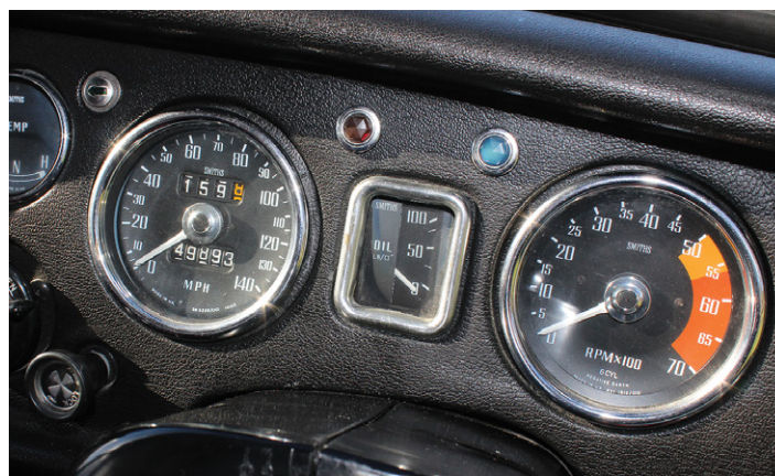
140mph speedo for MGC. Tacho red-lines earlier than on MGB.
